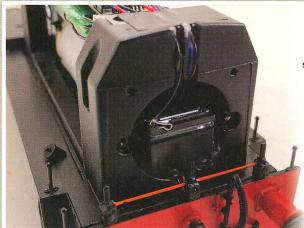
To provide a secure but flexible mounting for the speaker we used Black Tack – a high tack version of Blu Tack – to hold the speaker in place in the well. If you don't have Black Tack the traditional high street Blu Tack will work just as well.
