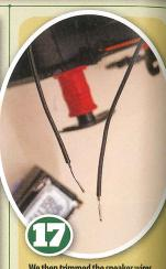
We then trimmed the speaker wires to the length required, removed around 6mm of the insulation again and tinned the bare wires to prepare them for soldering to the speaker connections.
