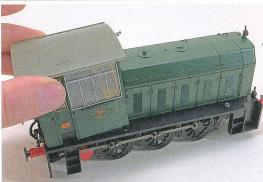
Once all the screws are out you can lift the cab section to allow the bonnet to be removed. Don't try to remove the cab straight away as it is connected to the main Printed Circuit Board (PCB) by a pair of wires.
