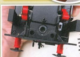
The remaining four screws are positioned at the four corners of the cab section. Two are at the rear at the outer edges. All are crosshead screws.
